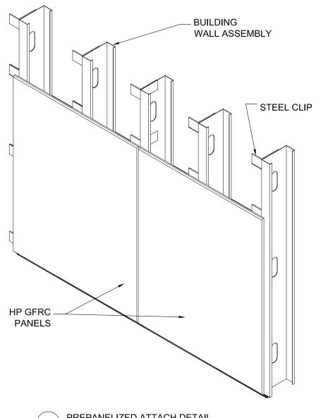
D4 PREPANELIZED ATTACH DETAIL NTS
